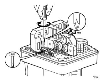
Fig. 4. Securing terminal block and label.
